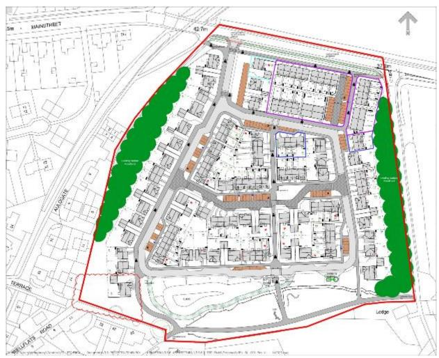
Fig. 5: Site plan from 21/03112/VAR4 showing the planned site layout. Note that the trees along the south boundary (W4, T1, T2 and T3) are not shown on this map.
